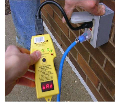
Detects difference in current between circuit wires
